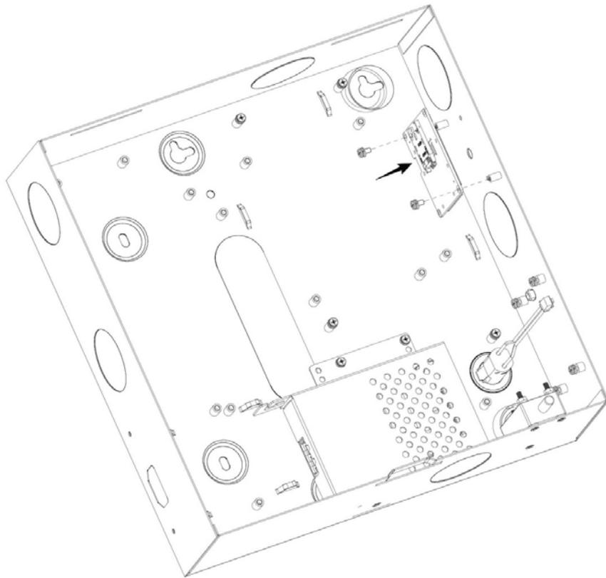
**Step 5** Secure the other end of the antenna patch cord to the antenna hole, and then install the external antenna on the hole.
