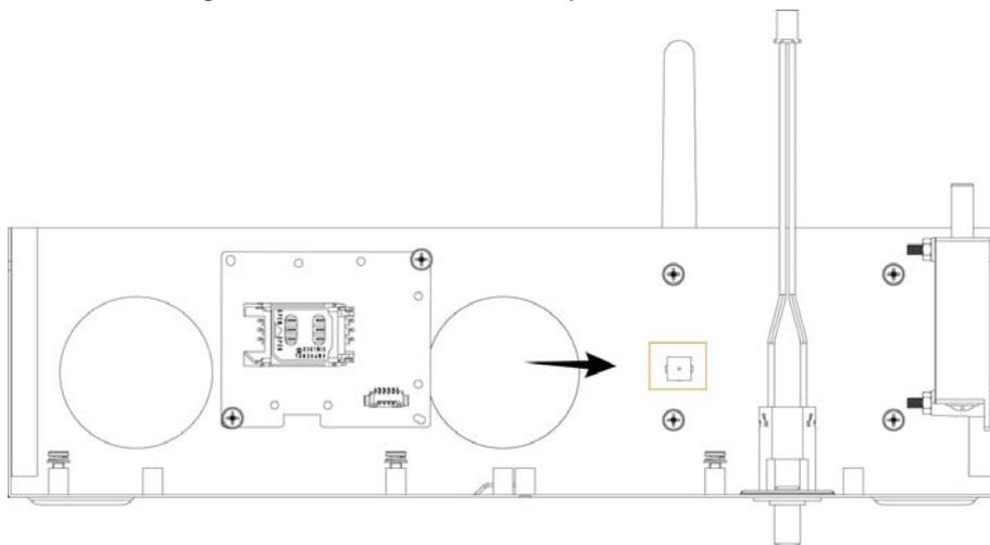
**Step 6** Connect the 4G module to the 4G port on the main board with the provided wire.
